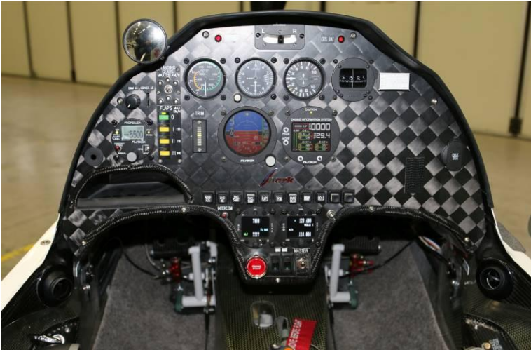
Standard instruments, electronic engine monitoring device MiniEIS, EFIS OBLO
